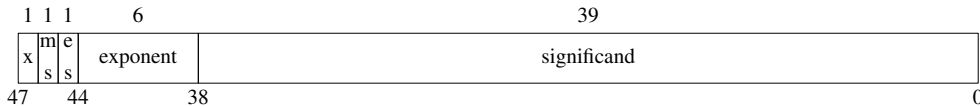
Figure 566.2: The Unisys A Series [1329] uses the same representation for integer and floating-point types. For integer values bit 47 is unused, bit 46 represents the sign of the significand, bits 45 through 39 are zero, and bits 38 through 0 denote the value (a sign and magnitude representation). For floating values bit 47 represents the sign of the exponent and bits 46 through 39 represent the exponent (the representation for double-precision uses an additional word with bits 47 through 39 representing higher order-bits of the exponent and bits 38 through 0 representing the fractional portion of the significand).
